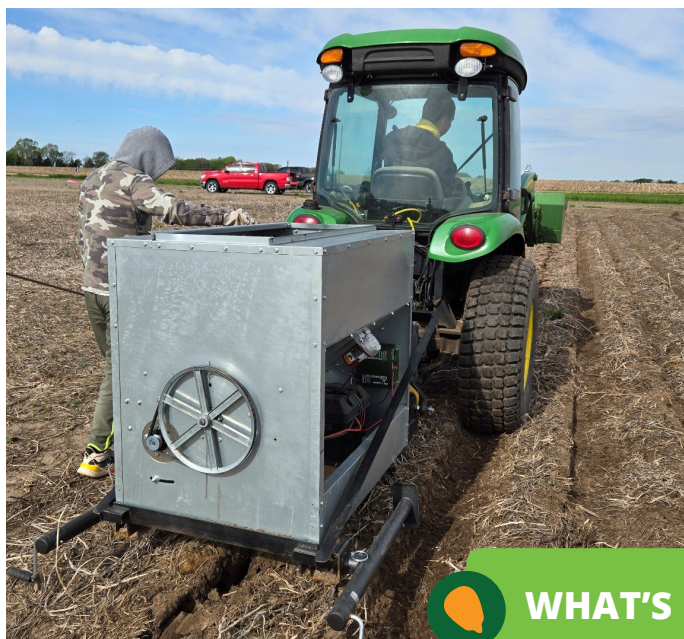
A feeder hopper and auger attached to a drop chute installed on a subsoil plow shank provided the means to inject 1500 lb/acre of locally sourced waste wood at a 14-inch depth.
