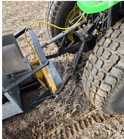
Figure 1. Auger shown injecting woodchips below the surface of the soil yields.
