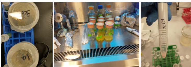
Figure 1. Some pictures of the research process: (a) microorganism propagation for fermentation experiments, (b) biosafety cabinet preparation for corn oil fermentation and (c) recovered cell pellet before PHA extraction.
